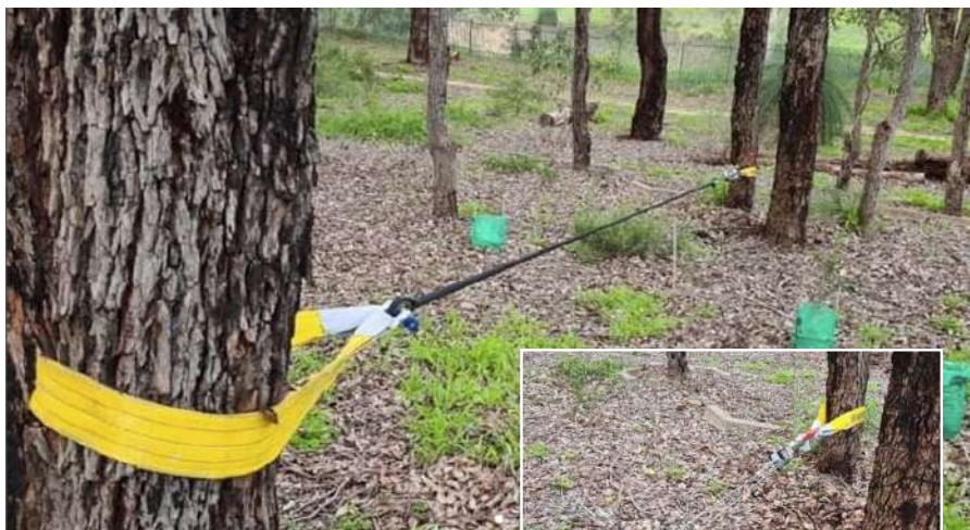
Tensioning to 2000kg using a come along and load cell
