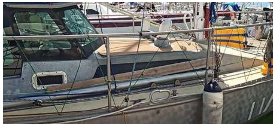
AVE's Yellow Central Lifelines, Tall Railing and Rope Lacing at Sandringham Yacht Club, Port Phillip
